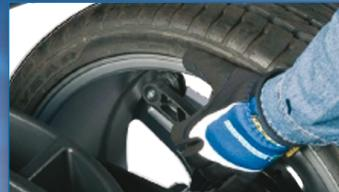
Technicians simply touch the rim with the gauge arm, and the system automatically enters the rim dimensions and selects the appropriate weight-balancing mode.
