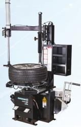
The turntable diameter scale markings allow operators to quickly and precisely position the jaws according to wheel size, speeding up the setup process and improving efficiency in high-volume environments.
