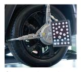
Clamp attaches to the tyre with limited clamping force without touching the rim for a safe, fast and consistent placement every time.
