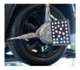
Clamp attaches to the tyre with limited clamping force without touching the rim for a safe, fast and consistent placement every time.
