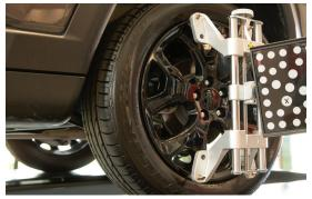
Fast and easy to use with self-centring design, two-sided claws provide reliable clamping, even over hub caps.
