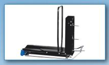
This lift helps facilitate the clamping of heavy truck wheels and offers ample storage space for cones, centring stars, and wing nuts.
